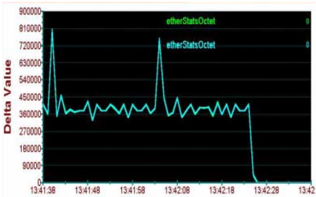
Figure 5: Drop in the number of bytes per second due to an application failure
